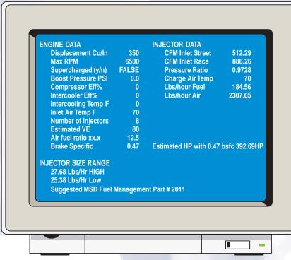
the engine's fuel requirements and electronic fuel injector size based on 12 engine parameters including:
